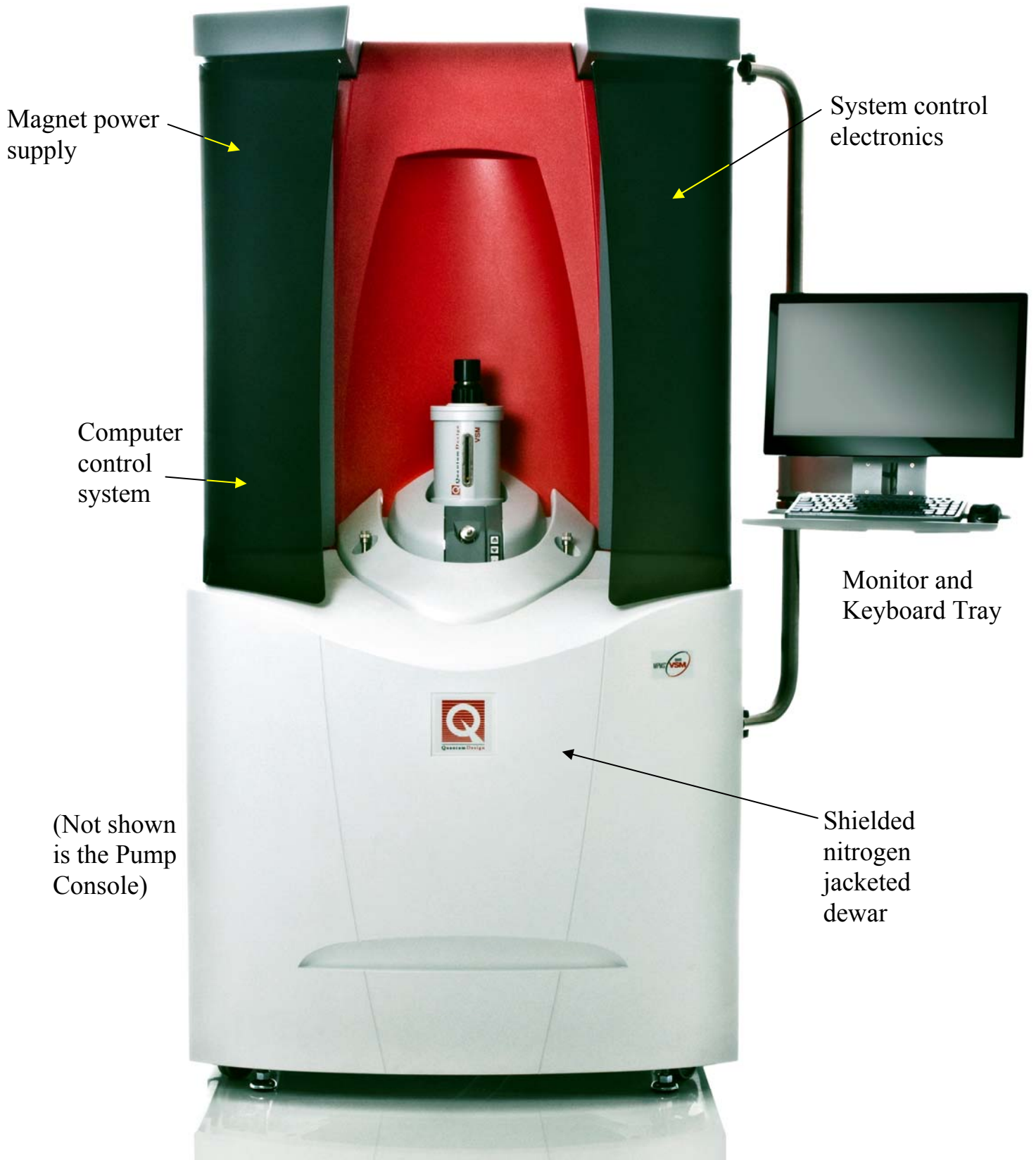
Photograph of an actual MPMS SQUID VSM at Quantum Design. Helium dewar is in the lower part of the cabinet and the computer and system electronics are in the upper half behind swinging smoked plastic doors.
